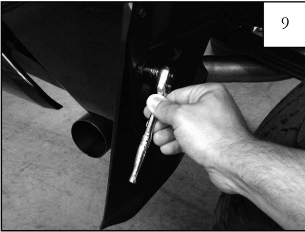
Using a socket wrench with a 10mm socket, remove second to top factory screw from mudguard.
