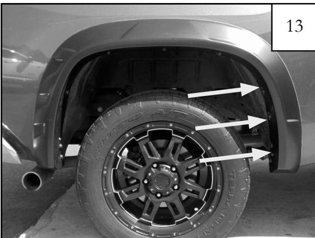
Using a 10mm socket, start three supplied 20mm Hex Screws through the forward-most holes of flare and into factory holes in fender.
