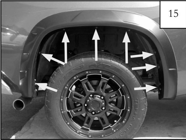
Ensure flare is properly positioned and tighten all screws. Installation complete. (See steps 16-17)
